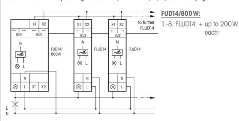
Capacity increase for additional lamps (☼:☼) in dimmer switch operating modes AUTO, LC4, LC5 and LC6. For operating modes EC1, 2 and LC1, 2, 3, see next page.
