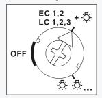
Capacity increase with capacity enhancers FLUD14 for dimmable energy saving lamps ESL and dimmable 230V LED lamps in comfort settings EC1, EC2, LC1, LC2 and LC3.
